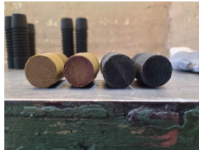
Figure 19. Bottom view of the shell cores from Shell Core Application #1, with zircon cores shown on the left and chromite cores on the right.
