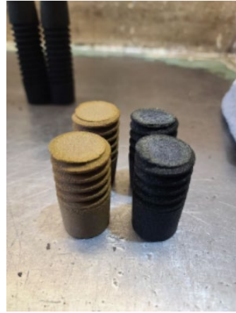
Figure 18. Shell Core Application #1, zircon cores are shown on the left and chromite cores on the right.
