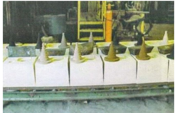
Figure 1. Prepared test molds and cores produced at UNI.
