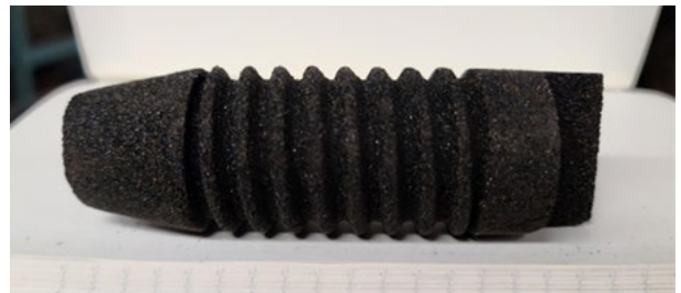
Figure 21. Side view of a chromite core from Shell Core Application #1.
