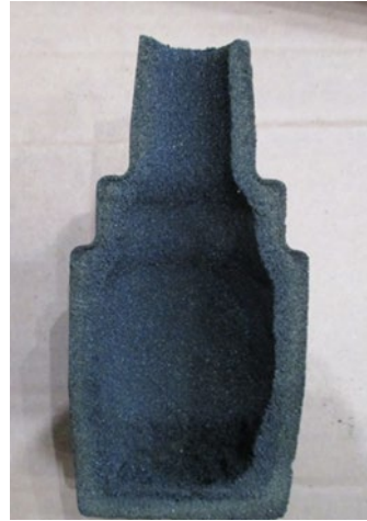
Figure 10. Case Study #1 shell core produced from the new blend.
