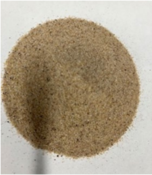
Figure 7. Case Study #1 historically used an 85/15 blend of lake/zircon sand.
