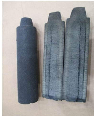
Figure 11. Case Study #1 shell core produced from the new sand blend.
