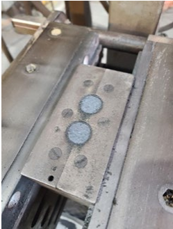
Figure 22. Tooling for Shell Core Application #2.
