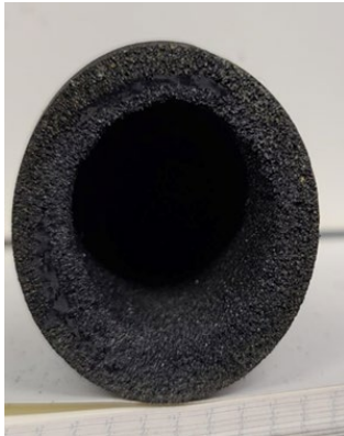
Figure 28. Bottom view of a shell core from 80 mesh chromite sand for Shell Core Application #3.
