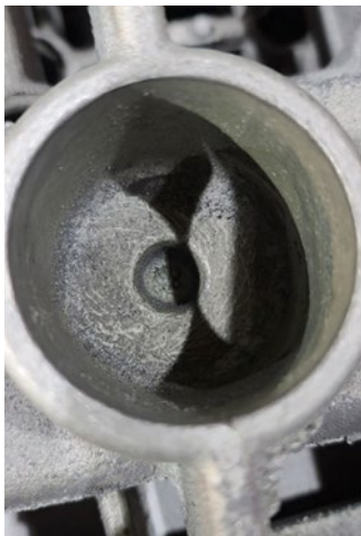
Figure 29. Casting used a shell core with 80 mesh chromite sand for Shell Core Application #3.
