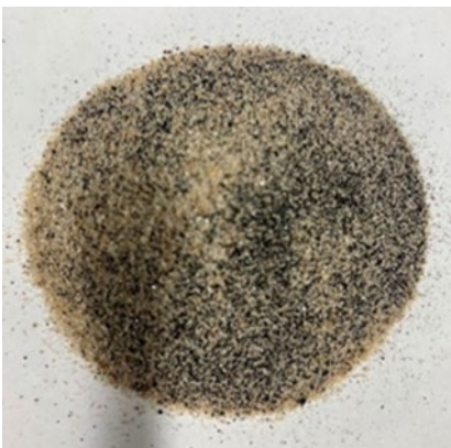
Figure 9. Case Study #1 introduced 50% of 80 mesh chromite sand and 50% of 60 mesh lake sand.
