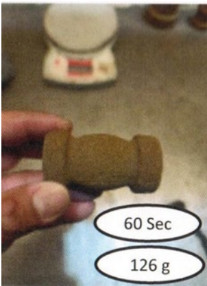
Figure 23. Zircon core production for Shell Core Application #2.
