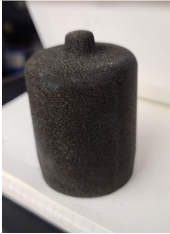
Figure 27. Side view of a shell core with 80 mesh chromite sand for Shell Core Application #3.
