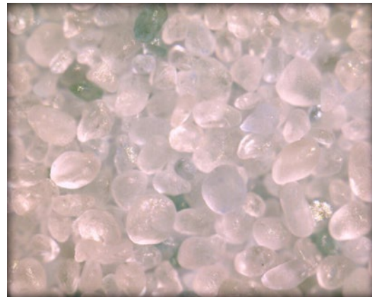
Figure 6. Case Study #1 historically used a blend of 85/15 lake/zircon sand.
